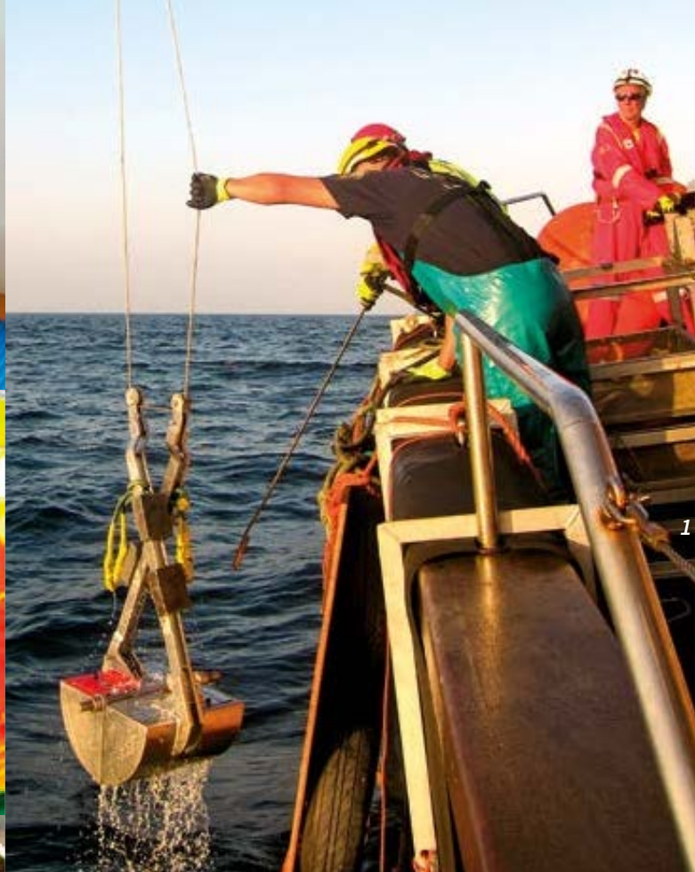
Van veen grab sampling done off R/V Angra Pequena (1), led by Fiona MacKay, with MSc student Sikhumbuso Maduna. Prior to grab deployment, substrate-type is verified by drop cam. Samples are washed on-board (6), revealing larger fauna such as the crab Macrophthalmus sp. from the Thukela shelf (2), the ubiquitous giant benthic foram Schizammia pinnata (3) and Amphipoda Byblis sp. (4) and Leucothoe sp. (5) abundant off Durban. These surveys are showing that unconsolidated substrates are very diverse and distinct assemblages are aligned with specific habitats. Also, amongst similar habitats, Durban is a distinct break in infauna distribution. Highlights so far are the 600 taxa that have been sampled and are under verification, several potentially requiring description. Surveys in some areas are a first for biological depiction of the KZN shelf, including in areas included in the proposed Phakisa MPA network. (Photos Fiona MacKay and Jean Harris).
