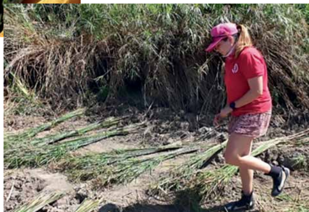
The material, imizi grass, used for durability testing in seawater and the development of the nature-based eco-engineered prototype structures.
