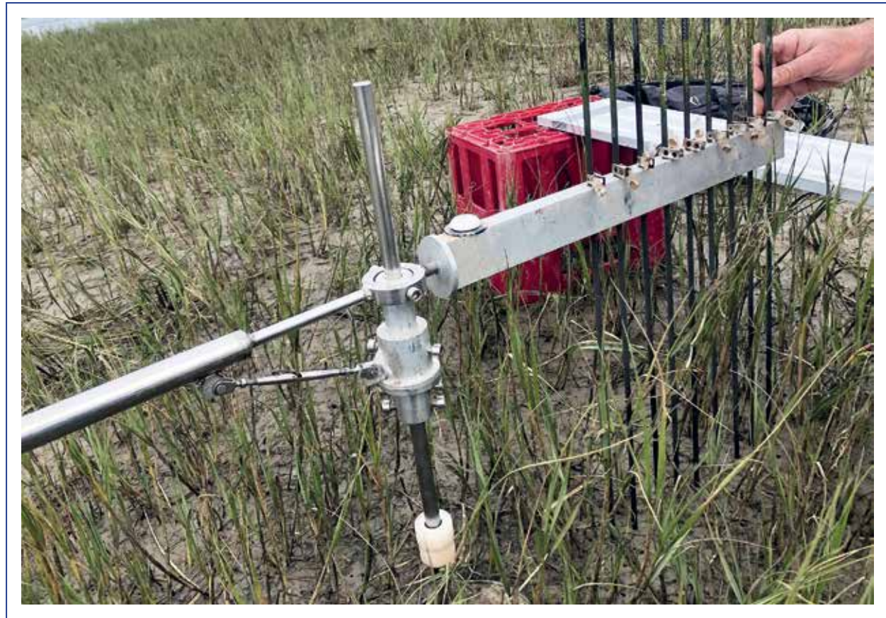
Figure 6.21 The RSET levelling arm that is attached to a receiver is used to measure surface elevations and can therefore monitor salt marsh level changes (Photograph: © Janine Adams).
