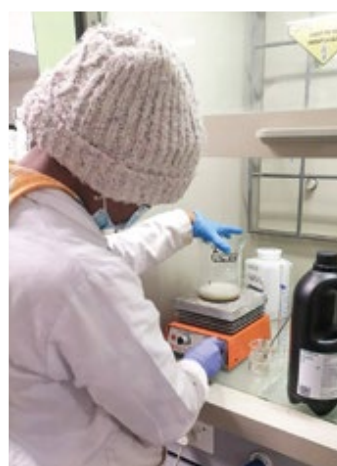
Left: In the laboratory, a student prepares sediment for sediment particle size analysis under a fume hood.
