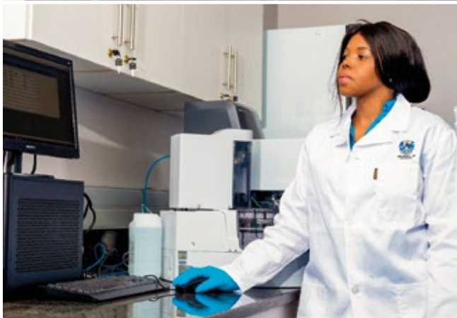
Three images to the left: The ICP-OES equipment and TOC analyser used to assess bioaccumulation of metals in water, sediment and animal tissues. Above: Lungelo Nsibande (PhD candidate) collecting sediment samples in Algoa Bay as part of his project assessing the macrozoobenthos community structure and sediment health status of Algoa and Cape St Francis bays in Eastern Cape.
