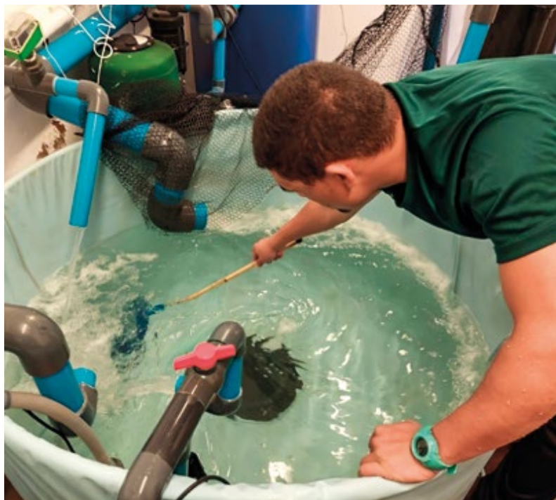
Bradley van Heerden fin-chasing a fish in the sump before placing it back into the respirometer to estimate maximum metabolic rate (MMR).
