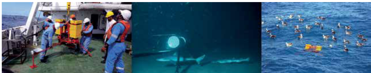
(From left to right) The crew of the RV Ellen Khuzwayo prepare the acoustic release stereo-BRUVs for deployment; species of dogfish (squalidae) and catshark (scyliorhinidae) approach the system while on the seafloor; prior to retrieval, the system floats on the surface signalling its position with radio and satellite beacons and drawing the attention of inquisitive seabirds.
