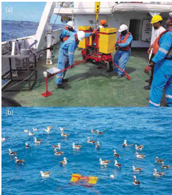
The untethered acoustic release stereo-BRUVs prior to deployment (a) and retrieval (b) during a research cruise to the outer Agulhas Bank.
