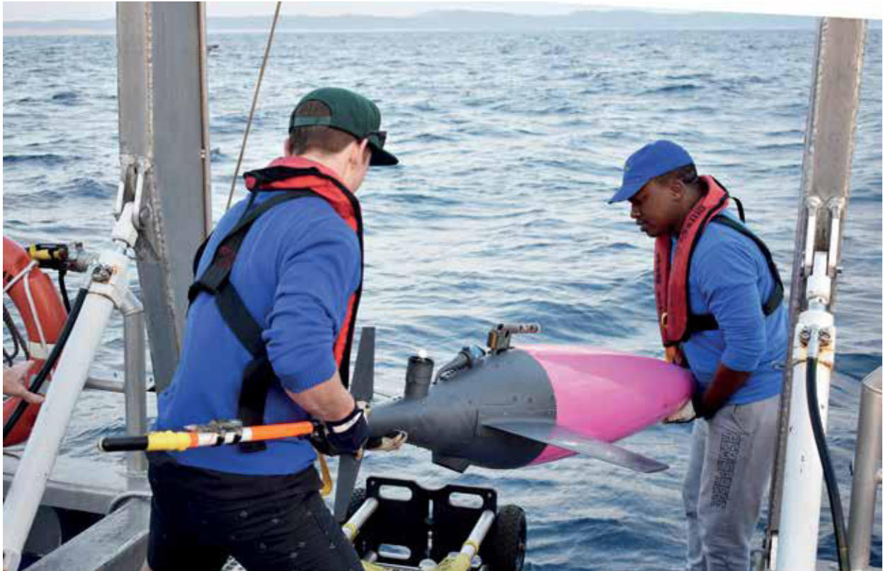
The deployment of a robotic sea glider on RV Phakisa .
