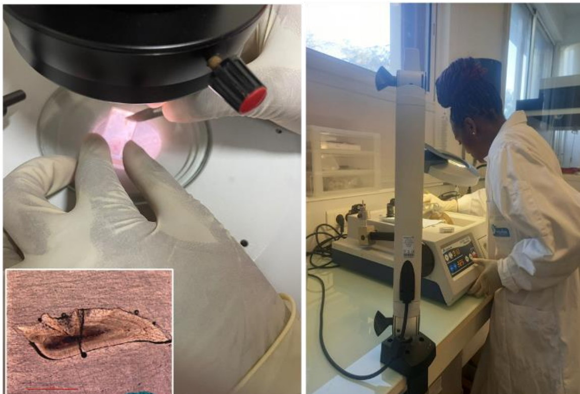
Figure 5: (a) A photograph of an otolith (fish ear bone) mounted on a glass slide prior to laser mass spectrometry; and (b) preparation of the sample for laser mass spectrometry.
