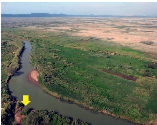
A river bank breach into the Link Canal brings large amounts of sediment-rich uMfolozi River water into the Honeymoon Bend area of the St Lucia Estuary during river flooding. This breach needs to be blocked as a matter of extreme urgency if Lake St Lucia is to retain its connection with the sea.
