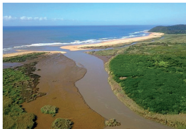
Extensive sedimentation in the St Lucia Estuary is clearly visible in this low tide aerial photo taken in 2023. These mainly compacted mud sediments effectively prevent the prevalence of a large tidal prism within the shallow estuary, and this therefore works against the retention and transport of saline water up the system.
